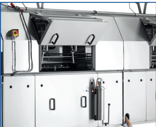
Two-phase door opening - cleaning position
