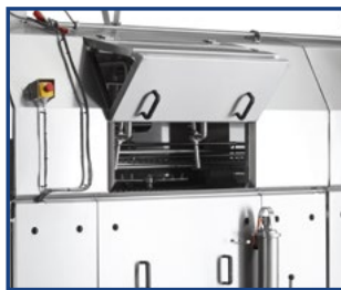
Two-phase door opening - cleaning position
