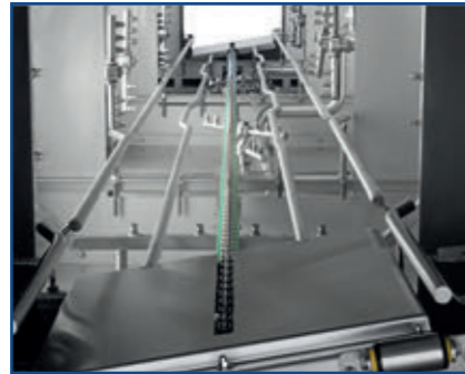
Image 17 Inclined / offset container guidance - no splash shadows
