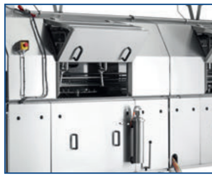
Image 25 2-phase door opening - drying position
