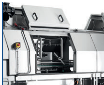
Image 24 2-phase door opening - cleaning position
