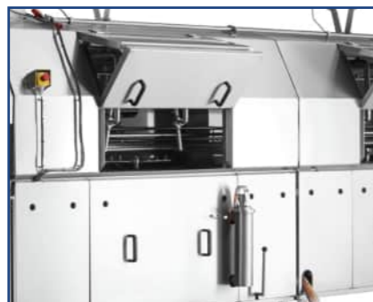
Image 15 2-phase door opening - drying position
