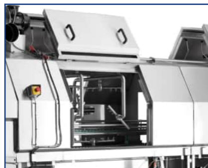
Image 14 2-phase door opening - cleaning position
