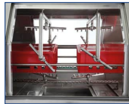
Image 17 Rotors of the cleaning zone
