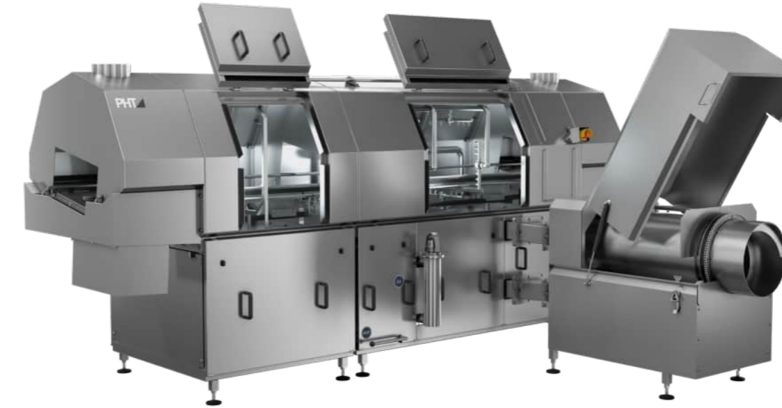
Image 18 Crate washing machine CM-series with drum filter, opened
