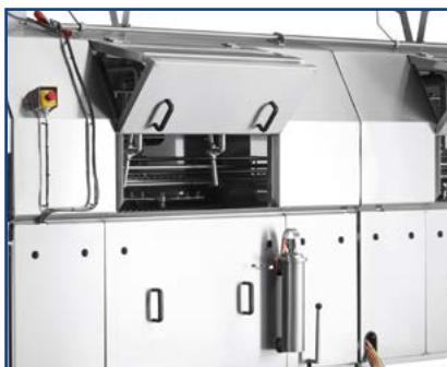
Image 15 2-phase door opening - drying position
