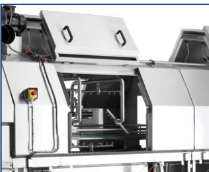
Image 14 2-phase door opening - cleaning position
